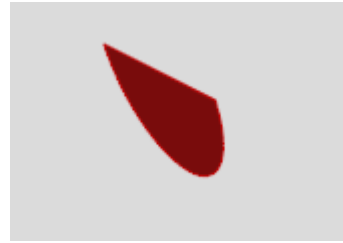
Semi elliptical crack
